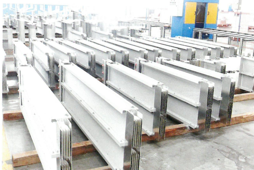
LCMC密集型插接式母线槽3150~6300A端面图 LCMC dense plug-in bus duct 3150 ~ 6300 A end view drawing
